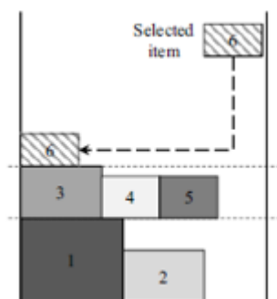
Example of an application of the next-fit decreasing height heuristic (NFDH). The numbers on the blocks are the order they are placed. Figure reproduced from Oliveira et al. (2016: fig. 8; CC BY 4.0).
